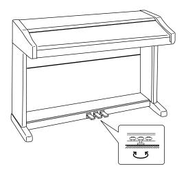
5. Turn the Adjuster (installed on the bottom of C) until it touches the floor to support the pedal board.
